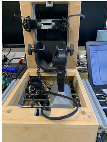
Figure 2. First prototype of the Ankle-PLAST with load cells, heel cup, and an automated ankle stress plate
